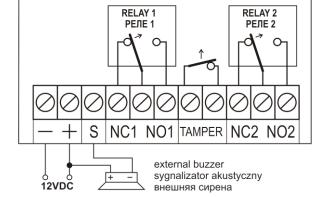
**IMPORTANT!** Output S must not be directly connected to (+) pole of power supply (see diagram above).
